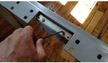
Insert teeth on cable tray into receiving slots on leg.
